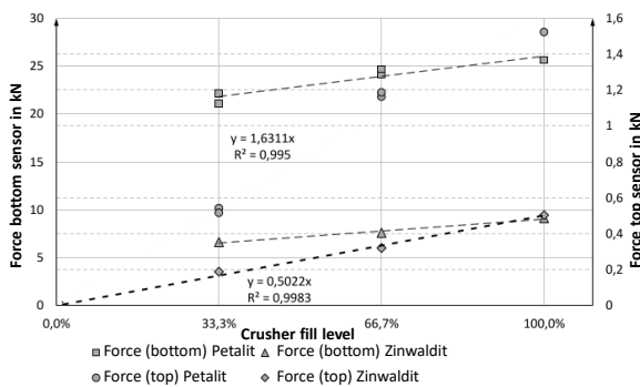
Figure 6. Change in crushing forces in the upper and lower regions of the crushing chamber as a function of the filling ratio for Petalite and Zinnwaldite, feed particle size: 15–30 mm
